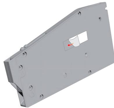
**STEP 2** - Fix the mechanism onto the cabinet by using the provided pins.
